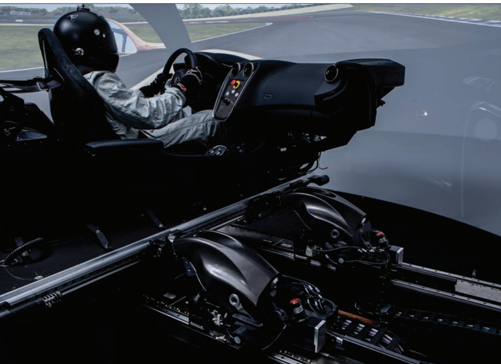
● Testing session in the vehicle dynamics simulator that features McLaren's motion algorithms
